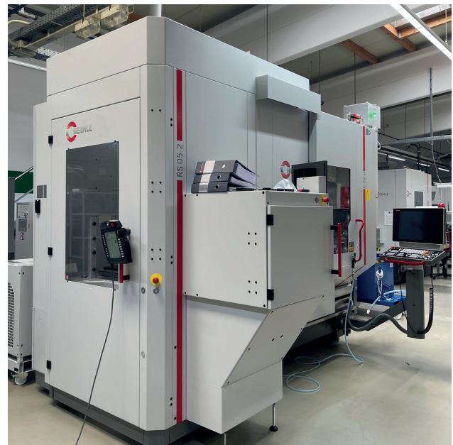
Figure 2: Hermle C22U CNC machine with RS-05 automation
