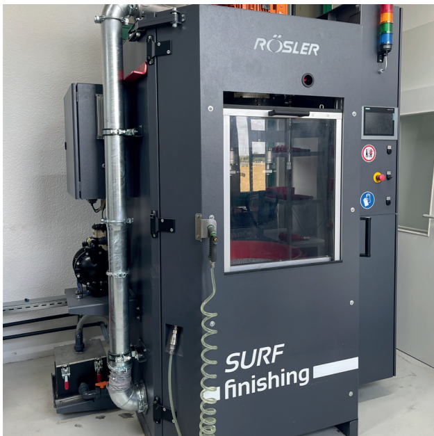
Figure 1: Rösler/R4/700SF drag finishing machine, semi-automated
